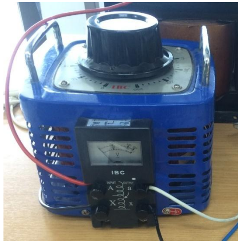
๕. Auto Transformer ( Variac ) 0 -250 V.
