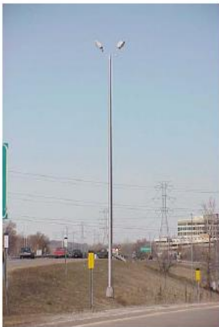
Double Vertical Mount Pole Arrangement (VMD-45)
