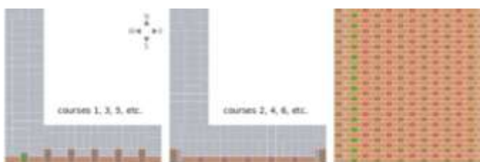
Double Flemish bond: two and a half brick
