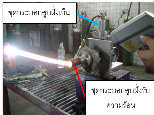
Figure 6 Experimental test of the artificial alpha type of small Stirling engine
