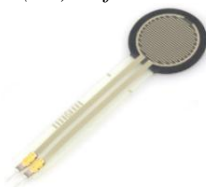
Figure 10. Force sensor or Force-sensing resistor. ( https://www.sparkfun.com/products/9375 )
