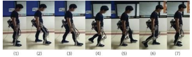
Fig. 8. Frame of step walking motion for data gait pattern generation.
