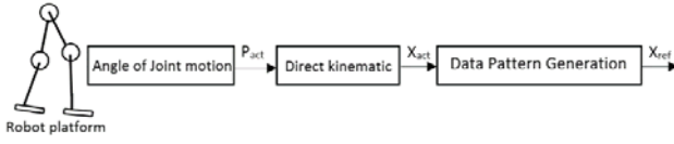
Fig. 6. The block diagram of data pattern generation
