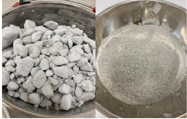
Figure 3 Crushed CLC (left); CLC powder size 0.25 (right)
