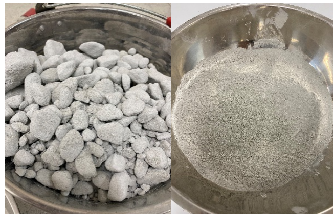
Figure 3 Crushed CLC (left); CLC powder size 0.25 (right)
