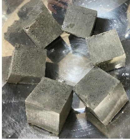
Figure 4 Cube-shape AAM at 24 hours after pouring into the mold.
