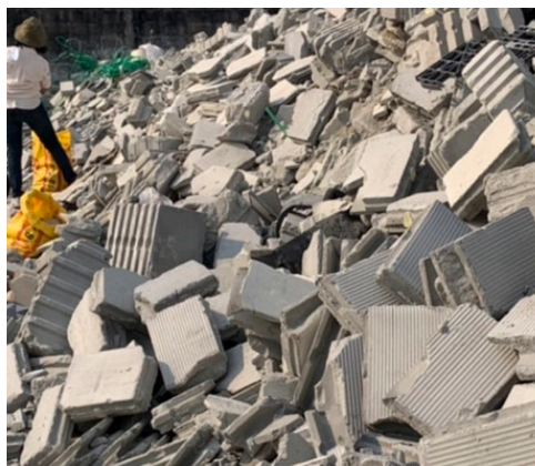
Figure 2 Broken CLC from manufacture
